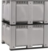
**Stackable:** The straight wall design allows the pallet boxes to be stacked one on top of each other, thereby saving floor space for storage or reduce empty transport costs. These kinds of bins can be stacked one above the other with or without a lid. The stacks are safe and stable due to the legs with self-locking wedges. Available with vented or solid walls. A drain is available on request.
